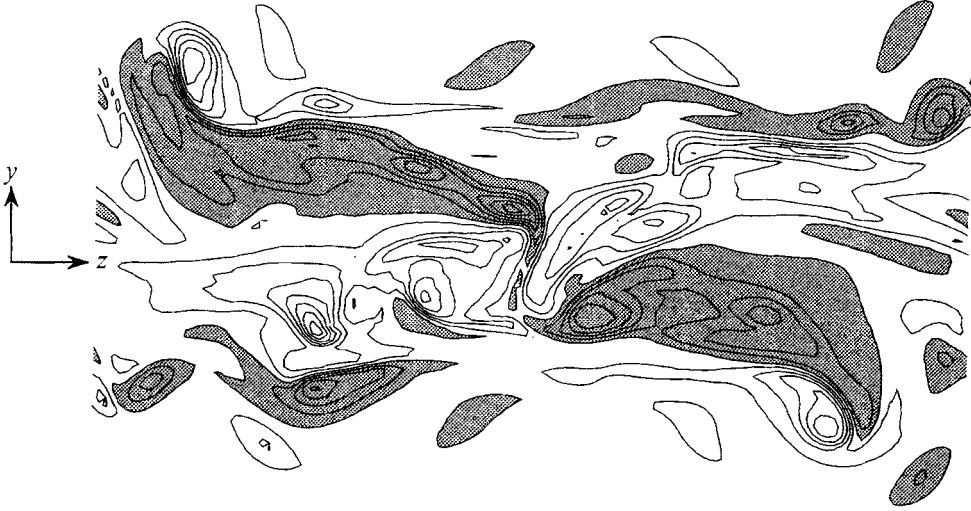
FIGURE 34. Recovery of a quadrupole meridional flow cell structure by t = 31.5 for simultaneous \text{CDI}_s 0.5 and \text{Trans } 1.0 evolution, reflected by \omega_z in a (y, z) -plane through the paired roll. Negative contours are shaded, and the contour increment is 0.3\Omega_0 .
